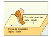
The friction force is contrary to the relative movement between the two contacting surfaces.
