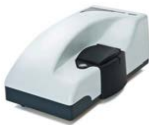
Figure 3.14. Zetasizer Nano ZS for particle size analysis.
