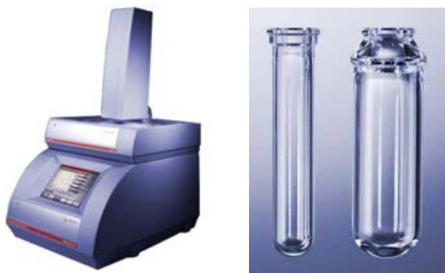
Figure 3.17. (Left) Anton-Paar Monowave 300 reactor and (right) borosilicate glass vials.
