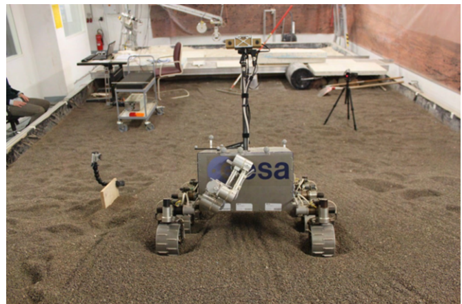
Fig. 7. ExoTeR at DLR performing a Wheel Walking test.
