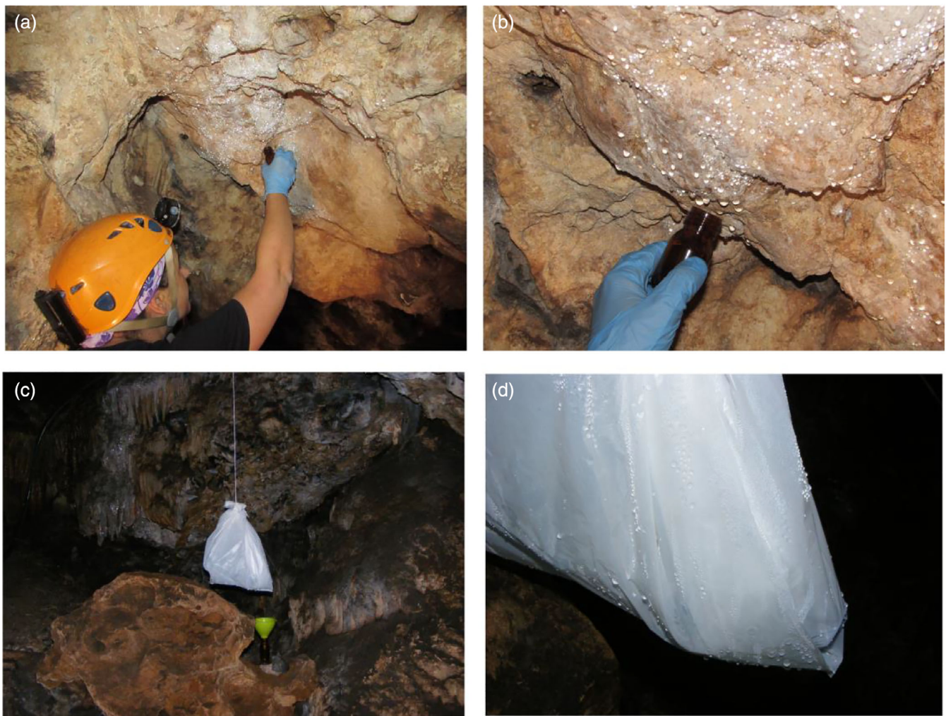
FIGURE 2 (a) Sampling of natural condensation water (Nw) in the ceiling of the area C2. (b) Detailed photo of the sampling method. (c) Device for sampling induced condensation water (Iw) in the area C3 and (d) detailed photo of water condensed on the ice bag
