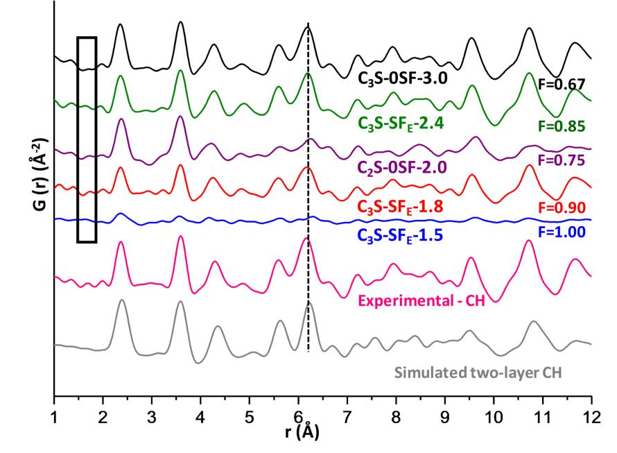
The PDF pattern for  $C_3S$ - $SF_E$ -1.2 can be used as a reference for C-S-H gel from alite hydration. Top seven patterns from ALBA. Data for synthetic C-S-H and C-A-S-H taken at Petra synchrotron, unreported. In collaboration with LMC-EPFL (P. Bowen).
