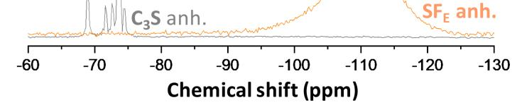
The signal situated at ~-110 ppm (SF), is negligible in all the hydrated pastes which proves that this phase has fully reacted at 4 month of hydration
