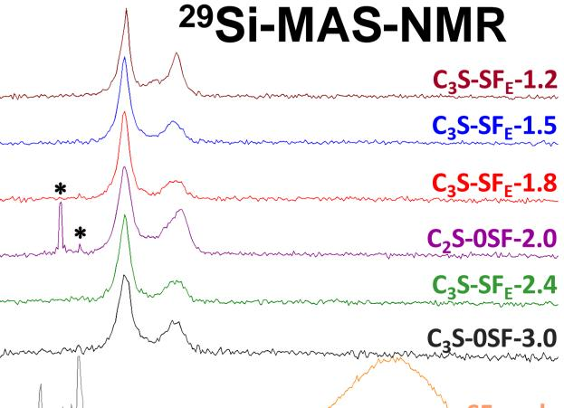
The C-S-H gel formed from the hydration of  $C_3S$  is composed by: - a defective clinotobermorite,  $Ca_{11}Si_9O_{28}(OH)_2 \cdot 8.5H_2O$ - stretched monolayers (or a few layers) of calcium hydroxide
