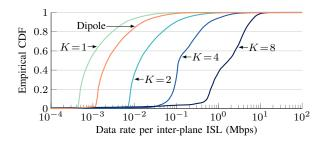
Fig. 2. CDF of the selected data rates per ISL with Butler matrix having  $K = \{1, 2, 4, 8\}$  antenna ports and a half-wave dipole antenna for  $\Delta t = 30$  s.
