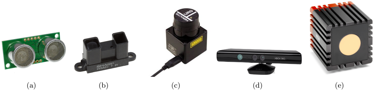
Figure 3.3: Images of range sensors commonly used in mobile robots (see table 3.1). (a) Devantech SRF05. (b) Sharp GP2Y0A02YK. (c) Hokuyo URG-04LX-UG01. (d) Microsoft Kinect V1. (e) SwissRanger SR4000.
