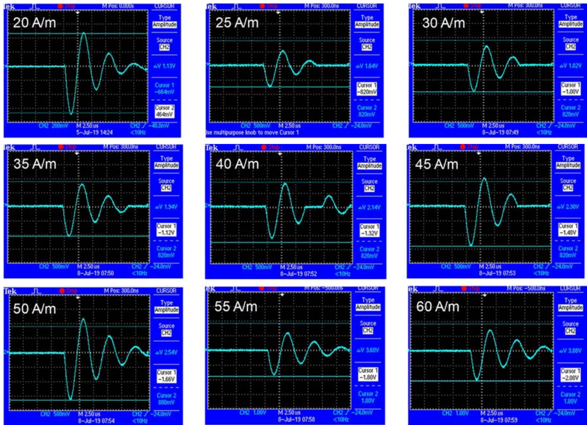
Figure 4.33. Applied waveforms for each current impulse level.
