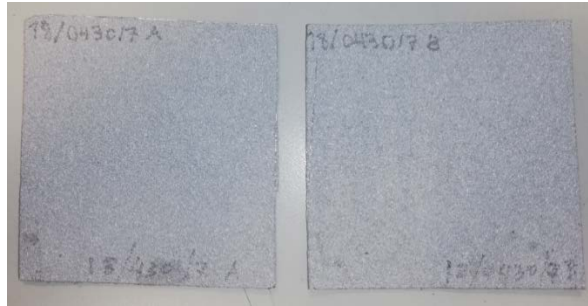
Figure 5.2. Example of schoop sprayed as sheets.
