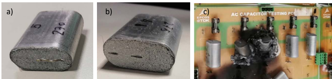
Figure 5.2.8.5. Appearance of winding failure causes: (a) broken wire, (b) desoldering of wire and c) melted windings.
