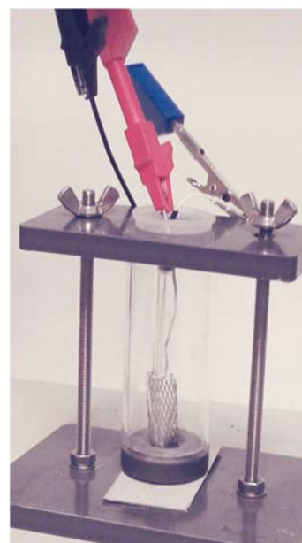
Figure 4.17. Set-up of electrolytic cell and the used three electrodes.
