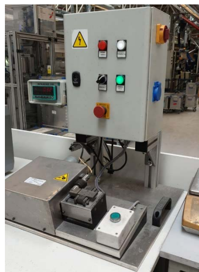
Figure 4.32. Set-up of mechanical test (tensile) on terminals with dynamometer model 9180 (Burster).
