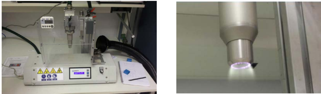
Figure 4.10. General set-up of atmospheric plasma by Plasmatreat GmbH (left) and detail of the Openair® Rotation jet RD1004 (right)
