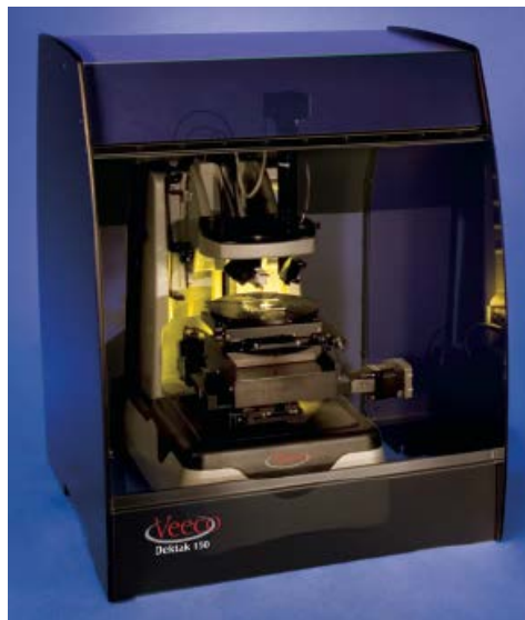
Figure 4.23. Contact Stylus Veeco Dektak 150 Surface Profiler
