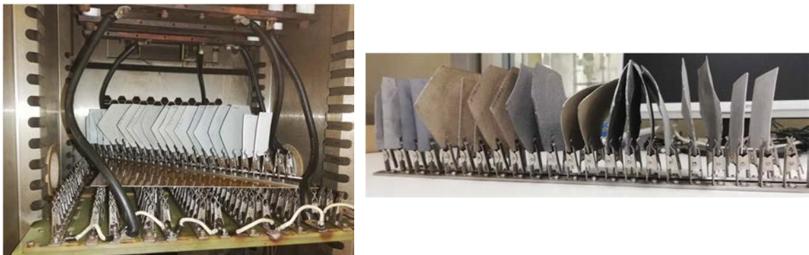
Figure 5.12. Schoop sheets before (left) and after (right) the aging application.
