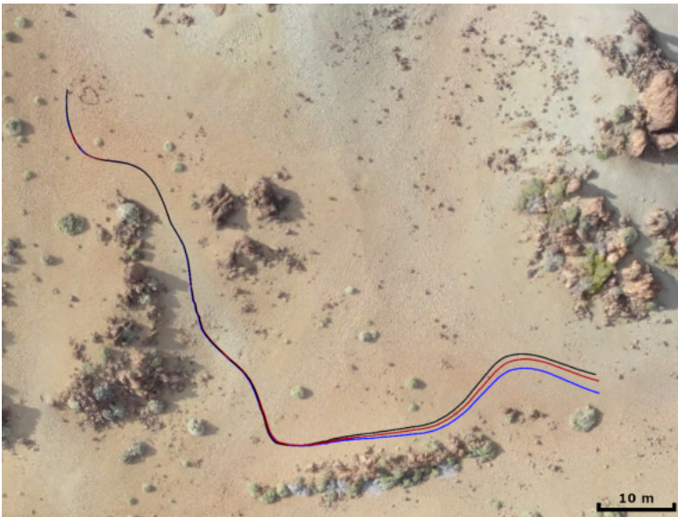
Figure 3.23: Traverses of experiments on relative localization. Black, blue and red lines represent the ground truth, odometry- and slam-estimated trajectories respectively.
