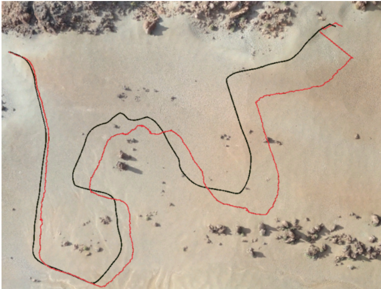
Figure 3.24: Orthographic views of the environment and the rover's traverses in it. The black and red colors correspond to the ground truth and SLAM paths accordingly. The pose correction is visible in the end of the traverse.
