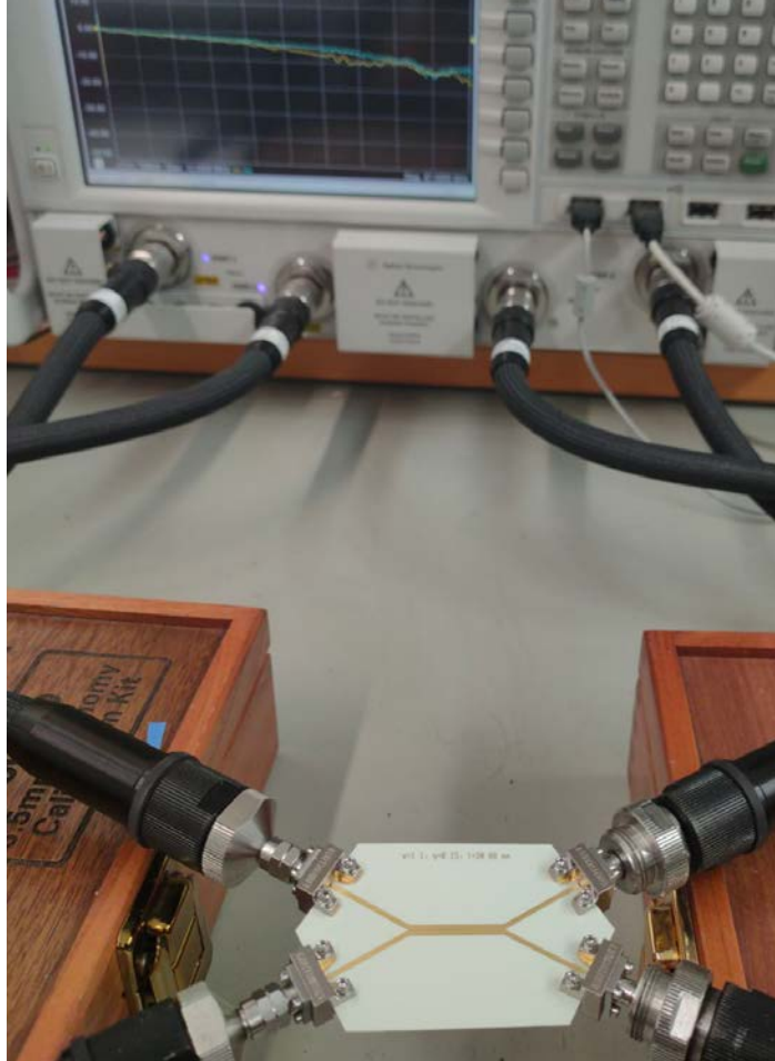
Figure 4.8: Photograph of manufactured coupled lines and the measurement setup using Vector Network Analyzer for Pure Mode S-parameters measurement.
