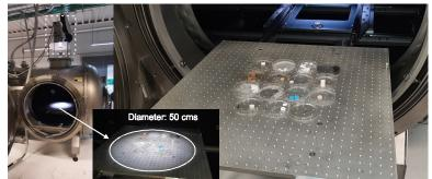
An halogen lamp and a optical diffuser installed in one of the upper ports of the TVC allow an homogeneous irradiation inside the chamber over a diameter of 50 cms. At full power, the irradiance at the targets is equivalent to that at Mars. The large irradiated area and the retractable rails allow easy loading of many samples to be simultaneously irradiated under specific vacuum and themperature conditions as shown in the picture.
