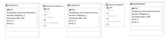
FIGURE 7.7: Initial IoT Palladio Resource Environment
