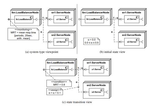
FIGURE 3.15: SimuLizar (a) System Type View,(b) Initial State View, and (c) Transition state view. (From Becker, Becker, and Meyer, 2013)
