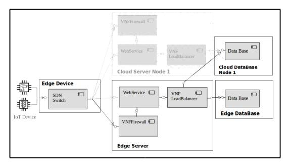
FIGURE 7.15: IoT Scenario Scheme 2 DB
