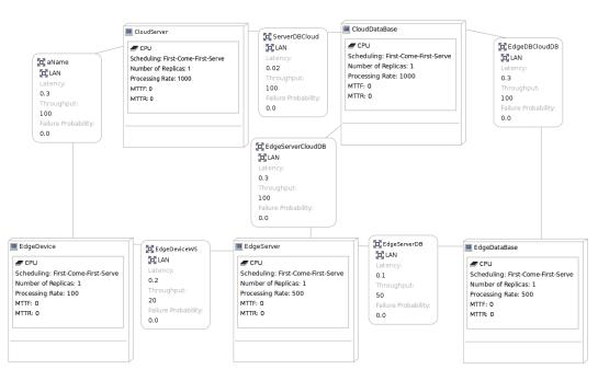
FIGURE 7.25: IoT Palladio Resource Environment Edge and Cloud
