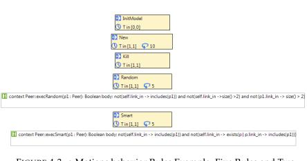
FIGURE 4.3: e-Motions behavior Rules Example: Five Rules and Two Helpers to Model the Behavior of the P2P Network System (extracted from *e-Motions Examples*)
