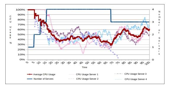
FIGURE 4.33: CPU usage correlation with the number of servers scaled: TW 10, TBA 5
