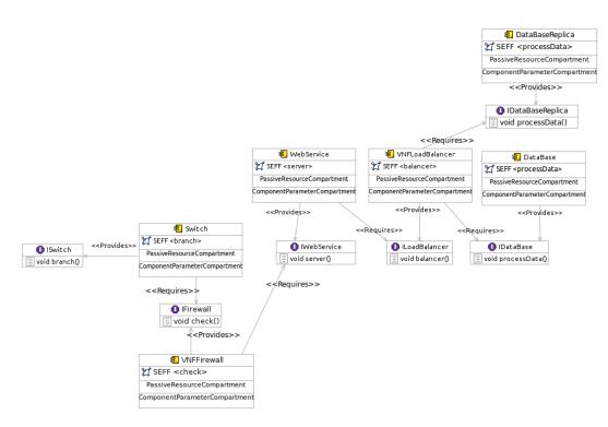
FIGURE 7.16: IoT Palladio Repository 2 DB
