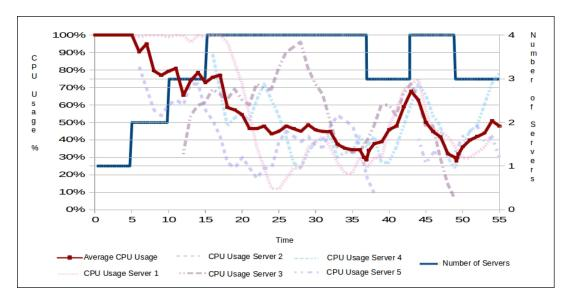
FIGURE 4.31: CPU usage correlation with the number of servers scaled: TW 5, TBA 5
