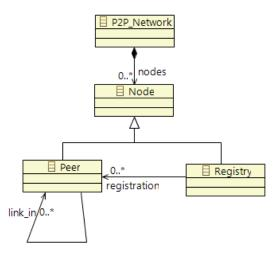
FIGURE 4.1: e-Motions Abstract Syntax Example: a Reconfigurable P2P Network (extracted from *e-Motions Examples*)
