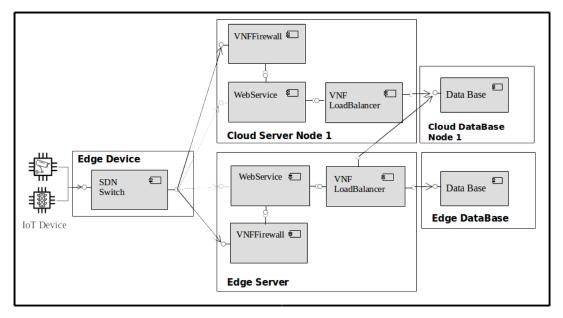
FIGURE 7.21: IoT Scenario Scheme Edge and Cloud
