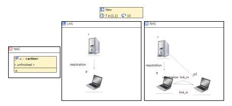
FIGURE 4.4: e-Motions Graph-Transformation Rules Example: The Rule Models the Creation of a new Peer in a P2P Network, Registers it, and Links it with an Existing Peer (extracted from *e-Motions Examples*)
