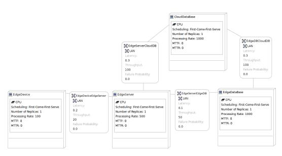
FIGURE 7.20: IoT Palladio Resource Environment 2 DB
