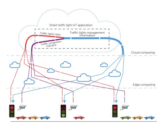
FIGURE 7.1: A high-level description of the smart traffic light IoT workflow application. Extracted from Nardelli et al., 2017
