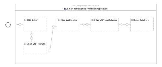
FIGURE 7.13: IoT Palladio Assembly Context with Firewall Edge
