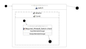
FIGURE 7.10: IoT Palladio Switch Branch with Firewall Edge
