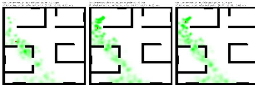
Fig. 3: Illustration of GadenTools accessing the gas concentration and 3D wind vector from a given Gaden simulation. By simply updating the robot position, the API provides the desired measurements.
