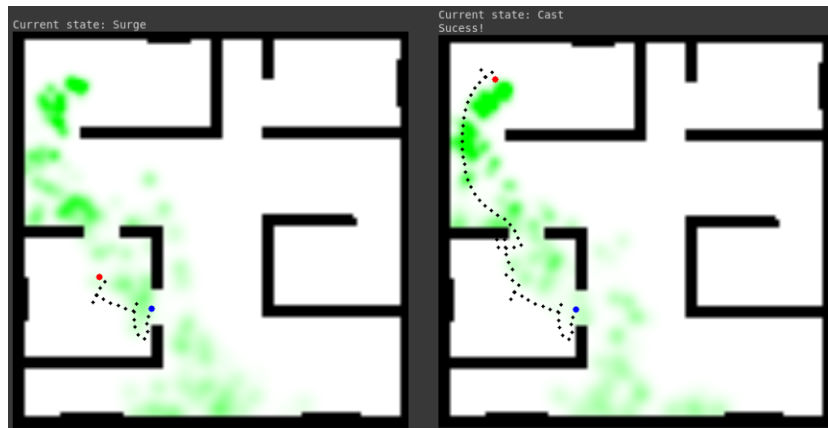
Fig. 7: An example of the proposed toolkit being used to implement an MRO algorithm. Pictured here is the Surge-Cast source localization algorithm. Both the algorithm implementation and the visualization are done fully in-notebook, and the code is presented to help users develop their own methods.
