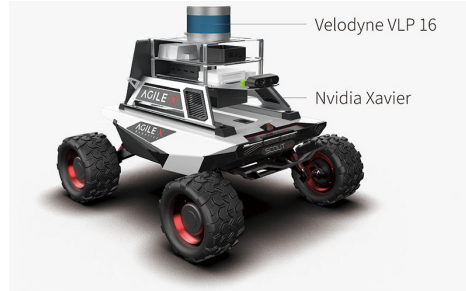
Figure 6.2: AgileX AI and mobile robot research kit.
