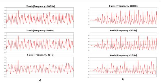
Figure 5.5: Raw data from accelerometer sensor of different activities: Walking (a) and cycling (b) at 100 Hz (top) and re-sampled data at 50 Hz (middle) and 20 Hz (bottom). It can be noticed that as the sampling rate decreases, aspects at high frequency are removed from the wave.
