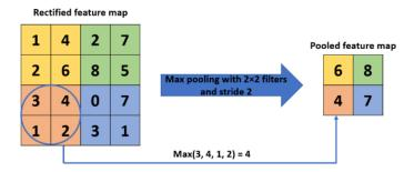
Figure 2.6: Example of Max-Pooling operation. Figure taken from reference 125
