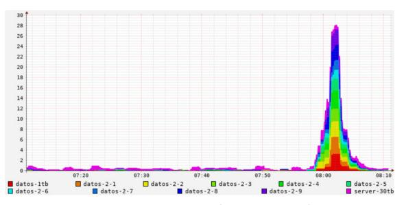
Figure 5.15: Load\_one. Number of threads per node (40 cores configuration). Plot captured from Ganglia cluster monitoring system for the master node (server-30tb) and 10 worker nodes.
