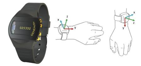
Figure 5.3: GENEActiv is a lightweight raw data accelerometer that allows for objectively continuous physical activity monitoring within clinical trials. Image taken and modified from [296].
