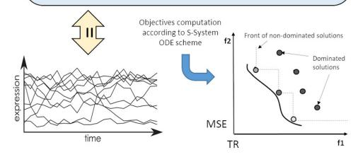
Figure 4.1: Graphical representation of solutions encoding/decoding withing the S-System setting process and the computation of the two objectives. The Pareto front approximation is constituted by using those non-dominated solutions obtained during the optimization process of MOPSOs.
