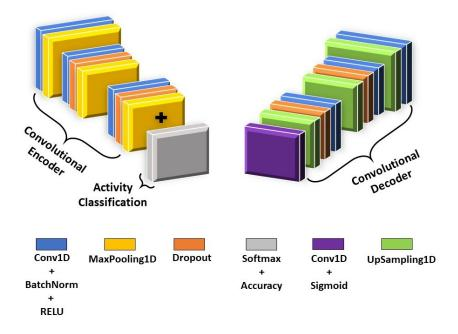
Figure 5.6: The proposed model contains an encoder part composed of three down-sampling blocks in the following structure [Conv1D + BatchNorm + MaxPooling1D + Dropout]. Moreover, each encoder layer has a corresponding decoder layer of three up-sampling blocks [Conv1D + Batch-Norm + UpSampling1D + Dropout]. Finally, the Softmax output layer is added for multi-class classification.
