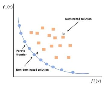
Figure 2.8: Example of a Pareto frontier for a multi-objective optimization problem with two objective functions.
