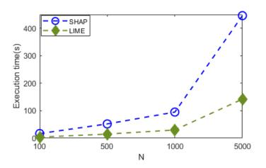
Figure 6.7: Efficiency of LIME Vs SHAP. Execution time versus N, where N represents the number perturbations in the case of LIME, and the number of samples for SHAP. Should be noted that LIME performs better than SHAP in terms of computational effort.
