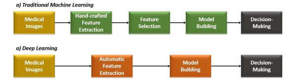
Figure 2.2: Artificial Intelligence workflow for image classification, in which traditional ML workflow includes hand-crafted human features. In contrast, the DL workflow provides a deep feature extraction to extract the most relevant features from images automatically.
