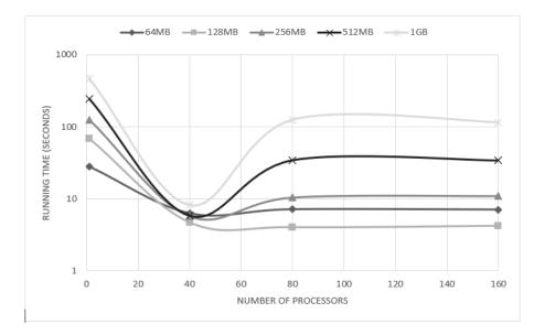
Figure 5.14: Running time in seconds (logarithmic scale) of the Spark Streaming process classification executed on 40, 80 and 160 cores in the cluster computing platform.
