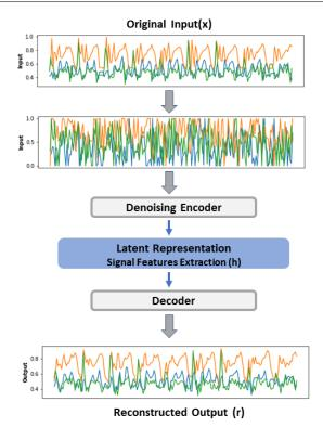
Figure 5.7: CNN Encoder-Decoder model. It contains a clean convolutional Encoder, noisy convolutional encoder, and a convolutional decoder. labeled and unlabeled data are processed by clean convolutional encoder and then corrupted with Gaussian noise. Then the convolutional decoder works to reconstruct the clean input(x) from high-level representation r = g(h).
