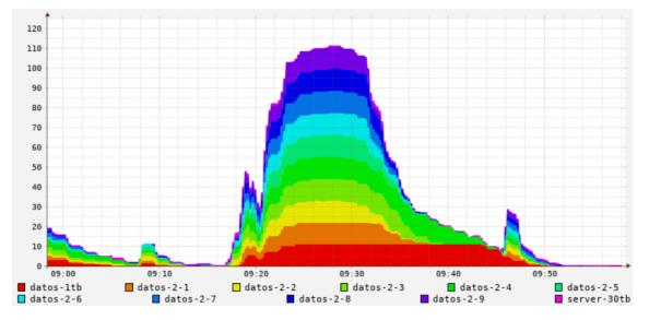
Figure 5.16: Load\_one. Number of threads per node (160 cores configuration). Plot captured from Ganglia cluster monitoring system for the master node (server-30tb) and 10 worker nodes.
