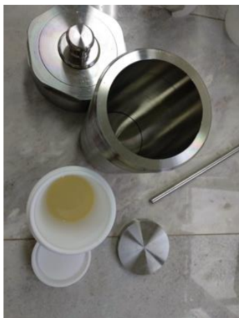
Figure 22: Teflon liner with DUT-4 solution after 24 h at 120 °C.
