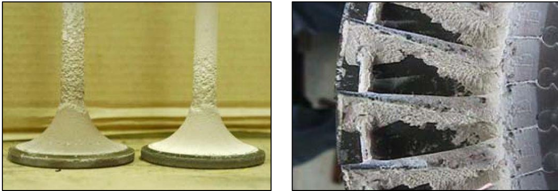
Figure 3: Exhaust valve and wheel of the turbocharger turbine damaged by siloxanes [18].
