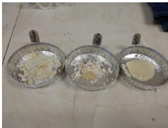
Figure 23: From right to left, DUT-4, DUT-4 (D) and DUT-4 (DH) after the DMF, DMF-DCM and DMF-DCM-hexane washes.
