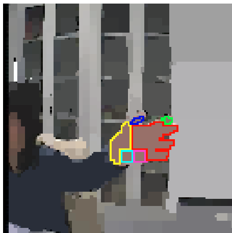
Figure 4.5: Segmented image using only the regular part of the BIP segmentation algorithm.
