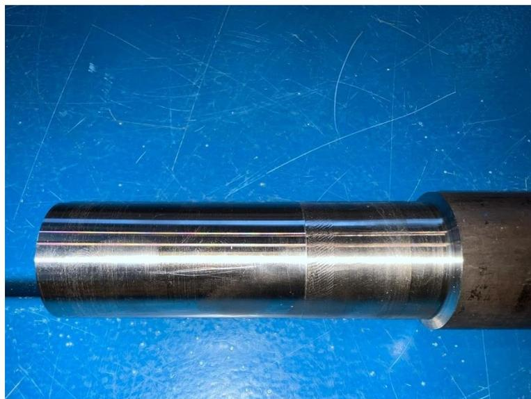
**Figura 100. Probeta AISI 1045.**
