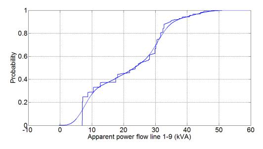
Figure 4.7: Cumulative distribution function for apparent power flow in line 1-9 Uncontrolled
