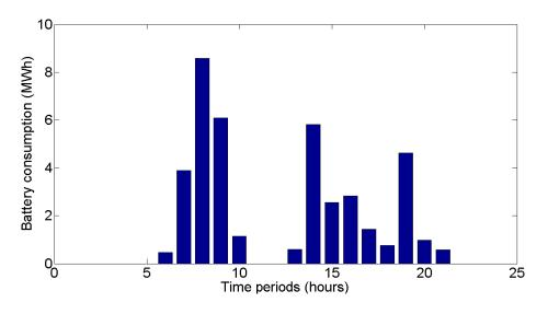
Figure 5.4: EV battery consumption in trips
