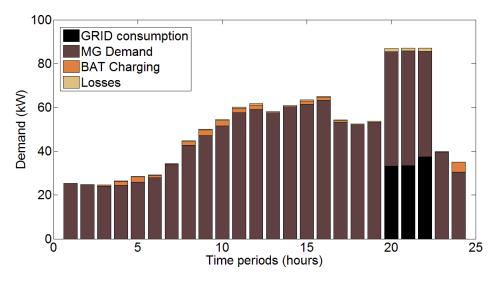
Figure 2.13: Microgrid power demand with DSM, k=12
