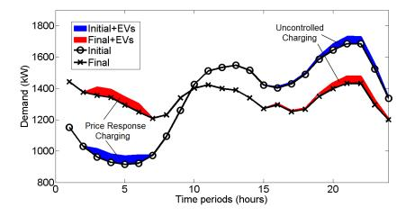
Figure 2.21: Daily electricity load curves with EVs charging
