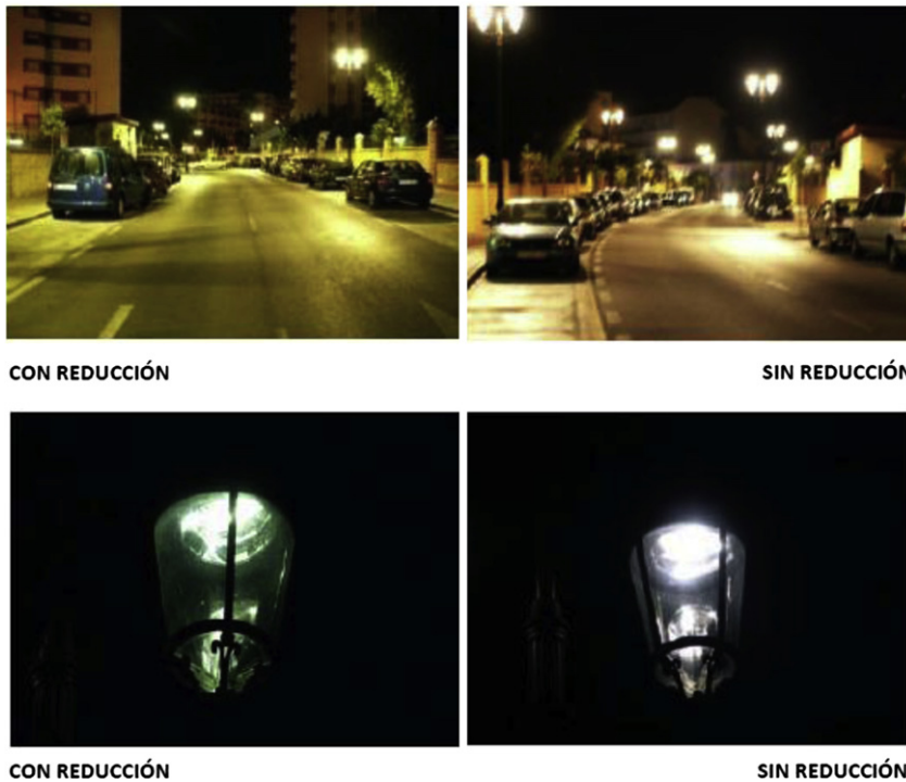
Fig. 4. Comparison of colour perception with colour balance. The photographs on the left use the electronic ballast for reduction.
