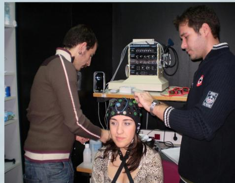
Data acquisition: four 8mm gold electrodes were placed next to C3 and C4 positions (10/20 international system). Ground electrode was placed at the FPz. Signals were amplified by a 16 channel biosignal amplifier (g.Bsamp) and digitized at 128 Hz by a 12-bit resolution data acquisition device (NI USB-6210). Projector 170 x 240 cm (115"). MATLAB programs were developed that allowed for both online and offline study. The statistical comparative study was performed in SPSS.
