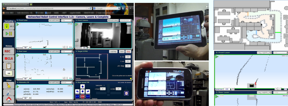
Fig. 3. Left and Middle) Our interface in a real remote driving experiment, running in three different platforms: a desktop PC, a tablet and a smartphone. Right-top) Simulated track (corresponding to one of our actual labs) where the experiments of this paper have been conducted. Right-bottom) One moment of the experiments where the robot goes out of the limits of the track, which is indicated to the user changing the color of the laser scanner sensor data.
